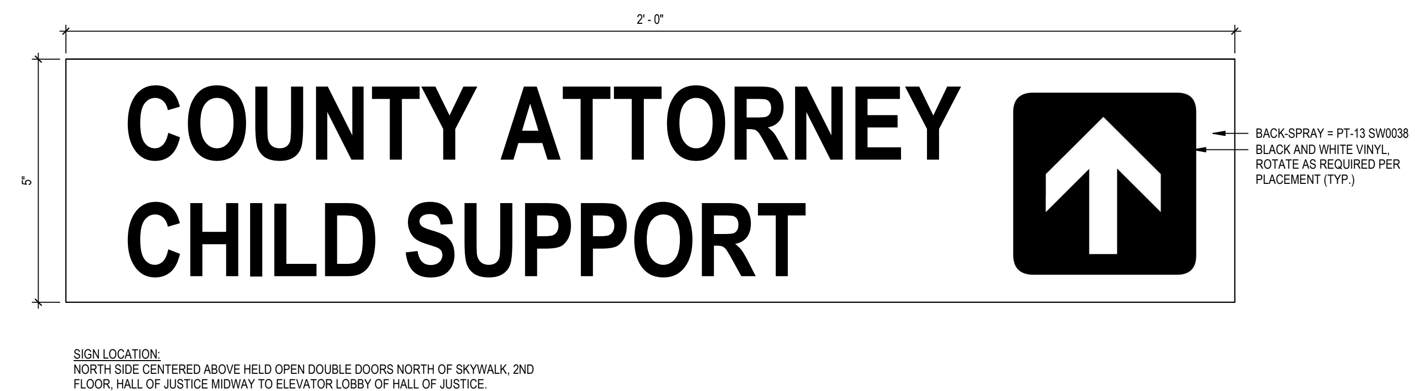
8 GENERAL WAYFINDING SIGN E5 SCALE: 6" = 1'-0"
